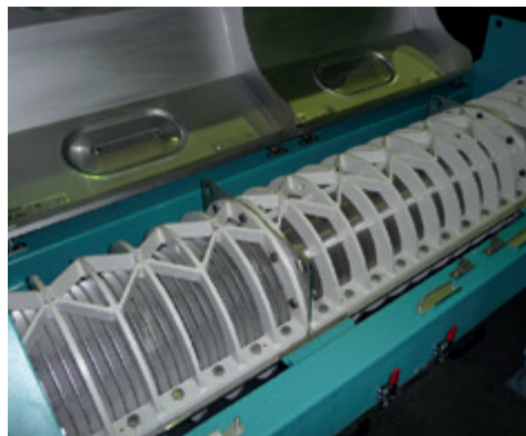
1 Entry area feed hopper / 2 Gear tooth coupling drive shaft screw / 3 Screening section with opened cover plates
