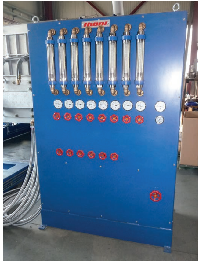
Cooling water control and connection unit with closed cooling water circuit
