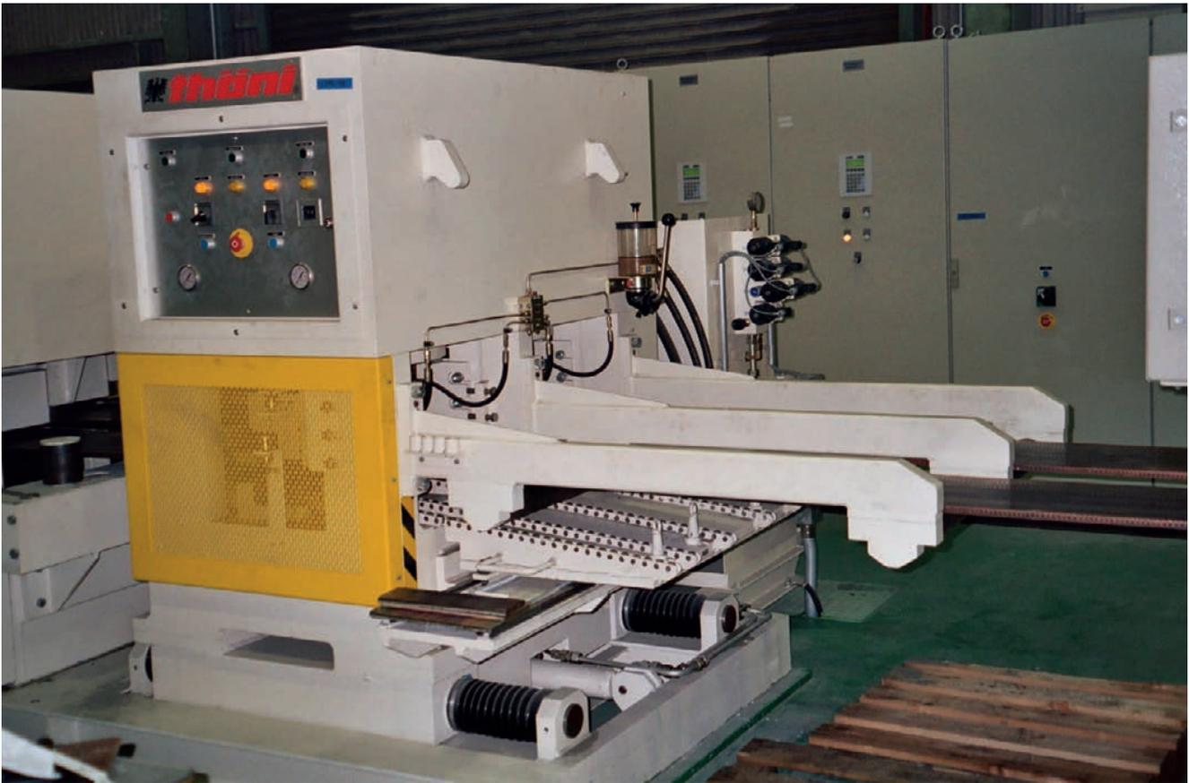
The pulse can also be generated manually. In that case, the cutting operation is also automatic. Scrap cutting with a minimum length of 300 mm can also be manual or automatic.
